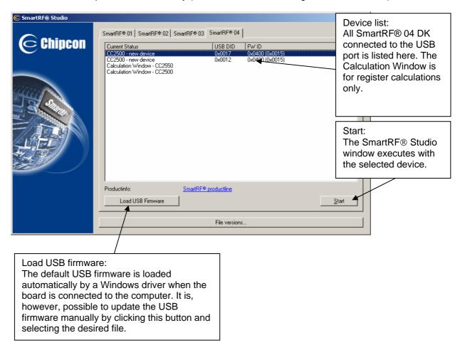
If a device is unplugged by accident or by intent while the SmartRF® Studio window is open, the window title will display "Lost Device". It is possible to reunite the device with the SmartRF® Studio window by right-double-clicking on one of them in the device manager, and then left- double-click the other.
