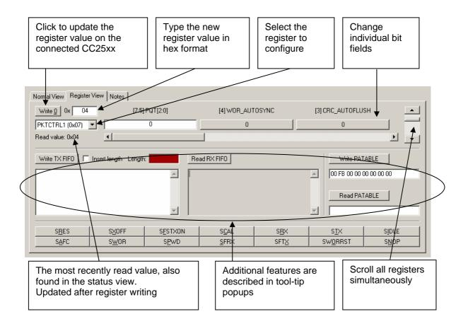
When the device has been configured properly, the command strobe buttons and the FIFO + PATABLE access fields can be used to operate the device.
