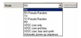
When Automatic power up sequence is selected, the CC102X wakes up in RX mode and check the carrier sense signal. The power up sequencing is initiated by a negative transition on PSEL. Pushing the 'wake up' button does this. Please refer to the data sheet for further information on power-on sequencing.
