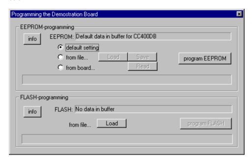
The interface communicates with the Evaluation Board. Before programming can start, you must plug the Demonstration Board into the edge connector on the CC400/900 Evaluation Board. The software will inform you if you have not installed the Demonstration Board correctly on the demonstrator before programming. Please see the User Manuals for the Development Kit for details regarding the Evaluation Board and Demonstration Board.
