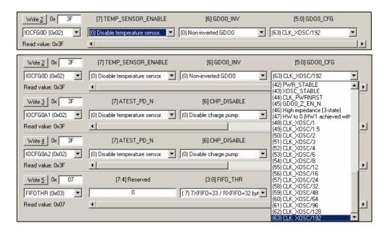
When temperature sensor is <u>enabled</u> and ADC test is <u>disabled</u> the CC25xx presents the correct parameter fields in a pseudo register called IOCFGA1:
