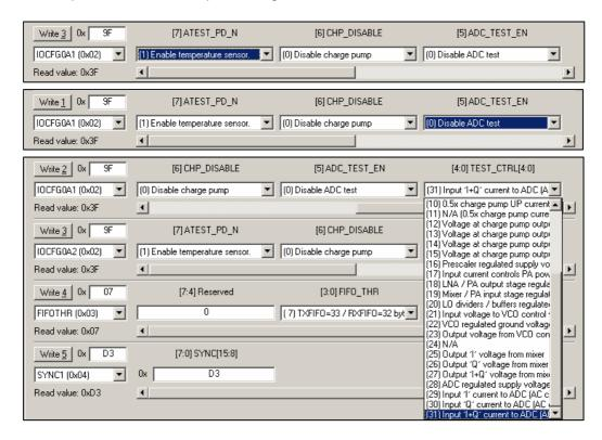
When temperature sensor is <u>enabled</u> and ADC test is <u>enabled</u> the CC25xx presents the correct parameter fields in a pseudo register called IOCFGA2:
