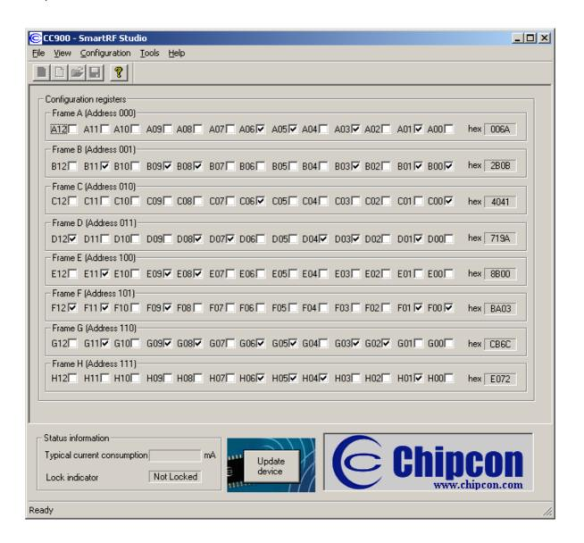
In this mode you can change the 13 different bits in the 8 registers directly by clicking on the white squares. These bits are used to program the transceiver chip on the printed circuit board (PCB) that follows Development Kit. We dissuade you to change the bits without contacting our company first.
