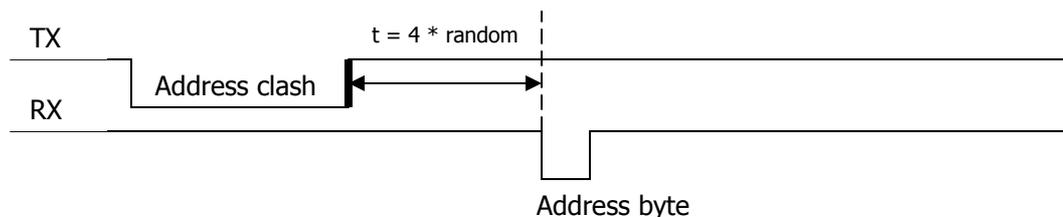
$t$  is measured from the end of the last TX stop bit to the beginning of the RX start bit
